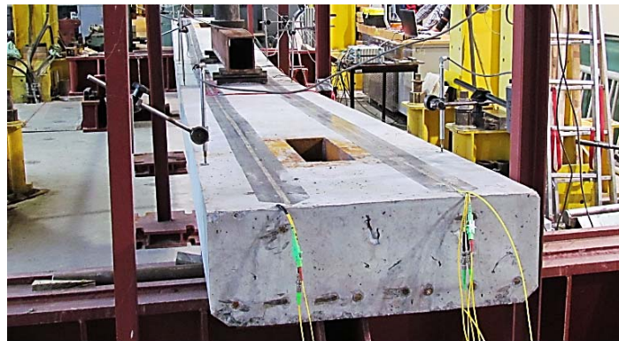
Figure 10. The view of examined platform during four-point bending test
