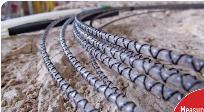
EpsilonSensor before installation in a lab specimen
