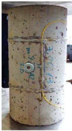
Fig. 4. View of the sample right before the experiment and a sample graph of the hoop strains in the time and distance domains
