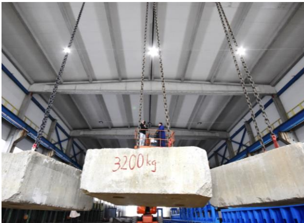
Figure 16. The view of smart girder during proof load test
