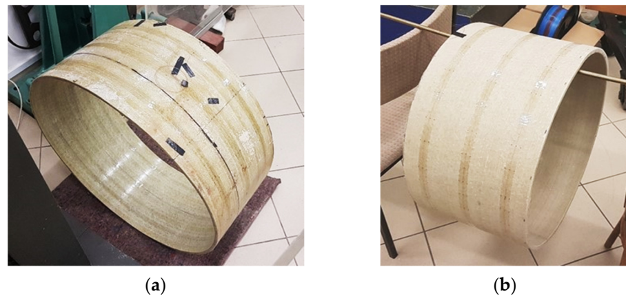
Figure 9. GRP pipe specimens prepared for testing: (a) DN 700 mm; (b) DN 500 mm.
