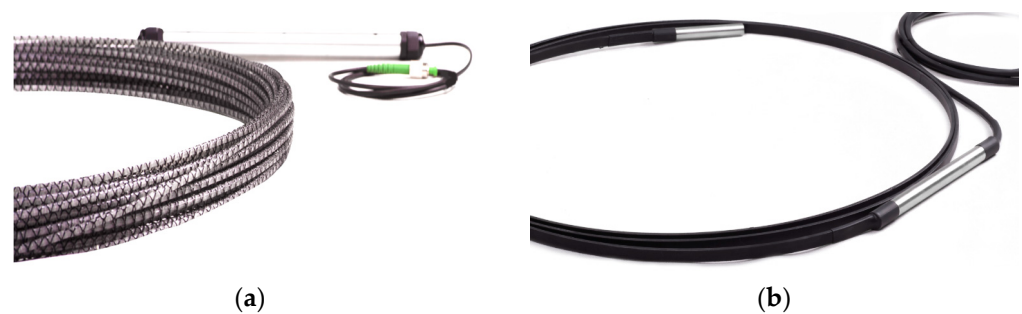
Figure 7. Examples of monolithic DFOS sensors for civil engineering and geotechnical applications: (a) EpsilonSensor for axial strains and cracks measurements; (b) laboratory version of 3DSensor for 3D displacement measurements [24].
